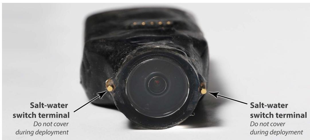
*Location of conductive terminals of the salt-water switch.*
